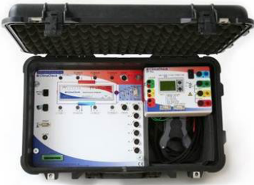
Figure 4. Field kit for Performance Analyser that does not require installation of flow meters to establish the performance and capacity.
